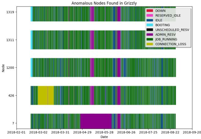
Fig. 3. The 5 most anomalous nodes identified on the Grizzly cluster over the 190 day period using an  $\epsilon$  of  $10^{-61}$
